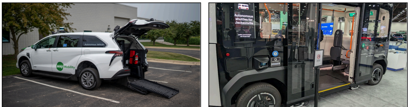
Figure 3: Examples of wheelchair-accessible vehicles (WAV). Left: May Mobility Toyota Sienna Hybrid BraunAbility upfit. Right: HOLON Urban WAV with a Q'STRAIT QUANTUM wheelchair securement system.
